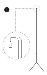
Mount the frame on the wall. Make sure the hook is fastened securely in your wall. Use an adequate wall plug or chose another hook if needed.
