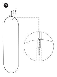
Secure the mirror. Make sure the hook catches the L-shaped screw on the back preventing the mirror from falling over.
